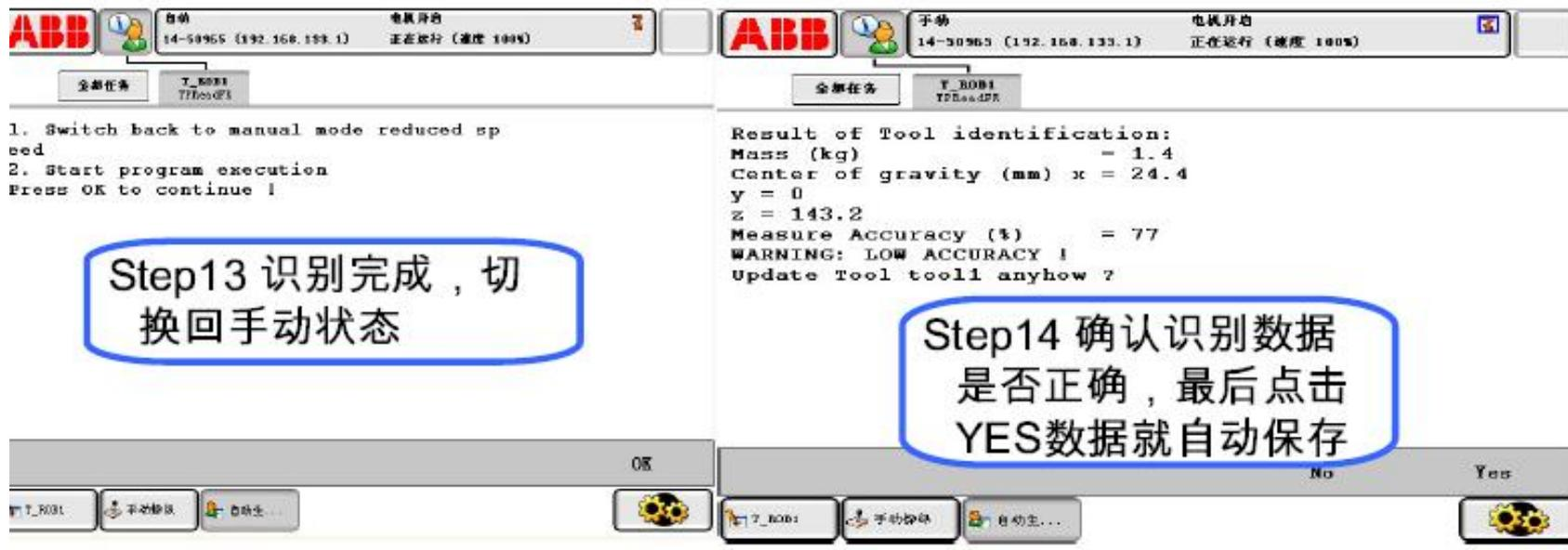
The screenshot shows two panels of the ABB robot control interface. The left panel displays instructions for switching to manual mode and starting program execution. The right panel shows the results of a tool identification process, including mass, center of gravity, and accuracy, with a warning for low accuracy. Both panels have blue callouts indicating specific steps.
